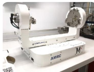
Smart Fixture with integral sensors and weigh scales
