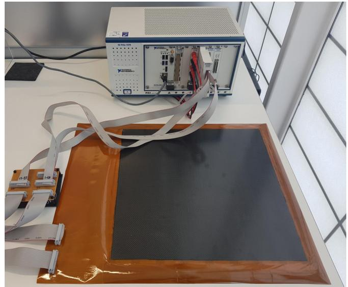
The initial test setup, showing the resistance data acquisition system and the flexible PCB embedded into the composite panel.
