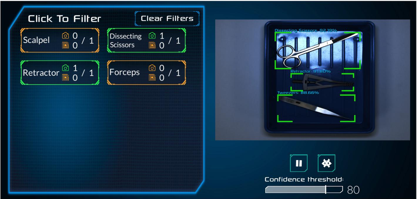
Figure 9: An example of the trained models being used to run a digital shadow board. The surgical tools are detected and compared against a previously made checklist of tools.
