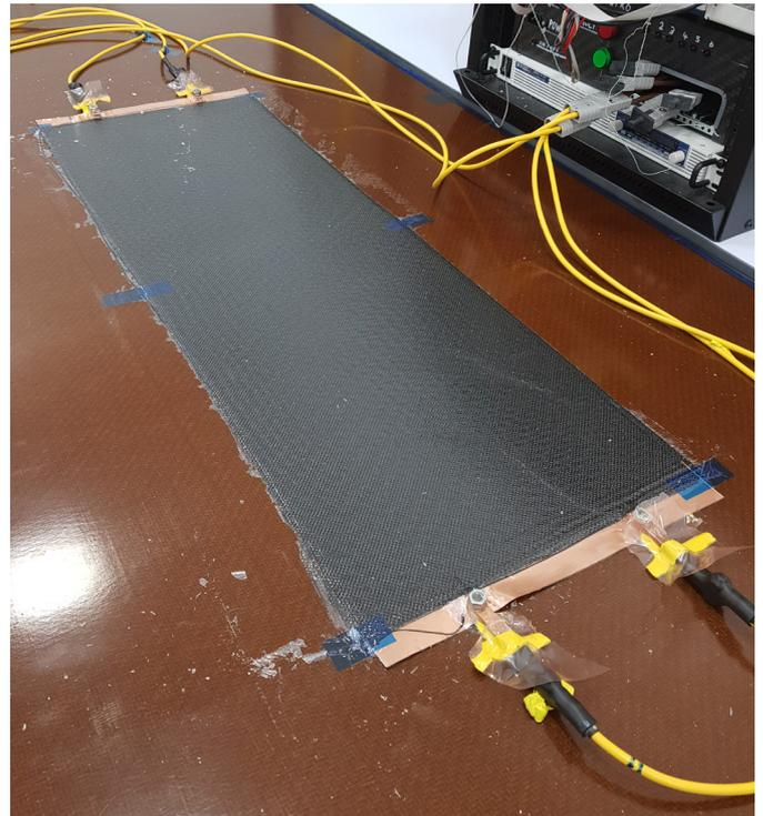
An example of the full electric cure setup, showing the copper electrodes in the component, connected to a computer-controlled power supply.
