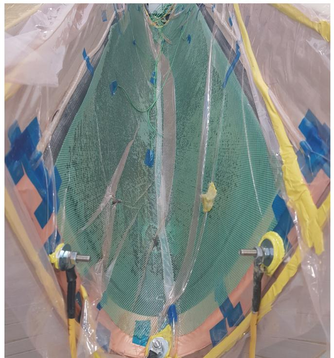
Example of the leading-edge demonstrator during the infusion and curing process, showing the electrodes required for self-curing.
