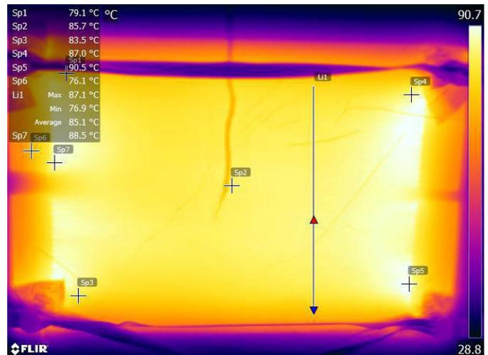
Infrared image of self-curing, showing the temperature distribution over the carbon fibre component during heating process.
