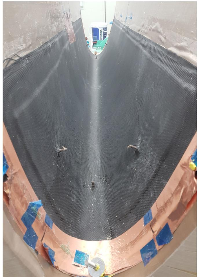
The final demonstrator after curing, once the manufacturing consumables have been removed.
