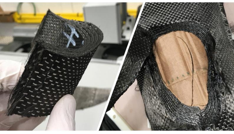
The ultrasonic knife was able to produce chamfered cuts (left) and complex pocket shapes (right) with high accuracy.
