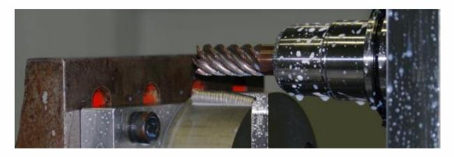
Technicut and Nikken worked together to develop optimised cutting systems for the high-speed machining of the toughest alloys.
