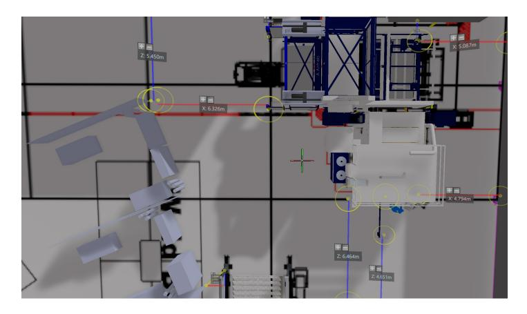
"We used a piece of software called Visionary Render to import the CAD files of the machines being installed which allowed us to put them in the right place by overlaying architectural drawings onto the floor plan of all the different components."
