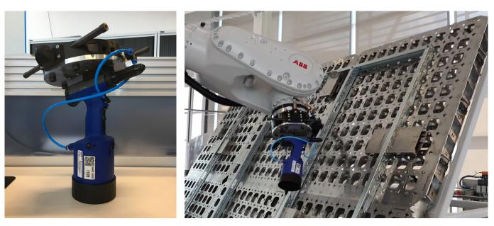
Figure 5. Gesipa Rivet Tool.
