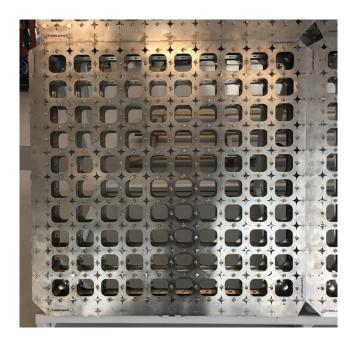
Figure 2. MetLase Pegboard Flexible Fixture.
